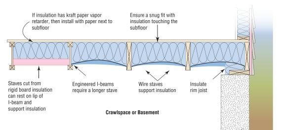
A stave is a mechanical method of supporting insulation from the bottom-up. Placing extra wire staves may be required to ensure adequate contact of the insulation with the subfloor even if it results in more compression of the insulation. Whether the insulation is oriented parallel or perpendicular to the rim joist, make sure the rim joist has full height coverage. Consider removable insulation to allow for pest and termite inspection.
