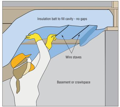
Air seal first if not done already. Wear proper safety attire and light your workspace. Plan and stage your work to minimize trips and be sure to measure your joist spacing to ensure you have the right length wire staves.
