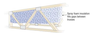
Consider using a spray foam insulation approach with web truss floor systems since the trusses provide a complex "puzzle" for insulating with batts.
