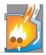
Gas log fireplaces should be a sealed combustion design because ventless gas fireplaces are unsafe.
