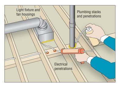
Any item that pokes through the building envelope is a candidate for sealing. Use caulk and spray foam for most applications.
