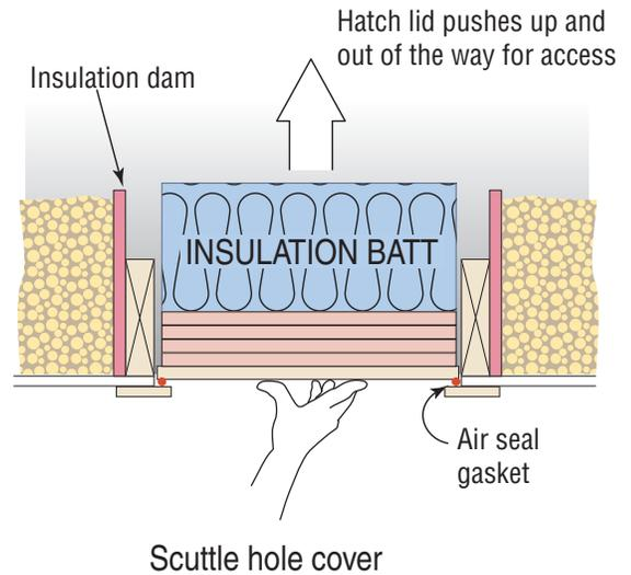
*Make cover box and scuttle coverings snug, yet with enough slack to allow for easy movement. Construct with rigid insulation board, nails, construction glue and duct tape. Insulation dams help to keep insulation in place. Consider installing a secure landing spot for movement in and out of the attic.*
