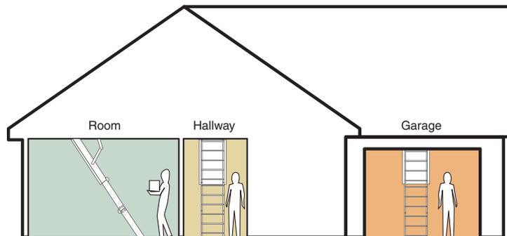
*Install an attic hatch/stair in a convenient location that provides ease of access. Follow manufacturers instructions for installation and plan how you will air seal and insulate this big hole in your ceiling. Attic access covers are essential; solutions range from factory-made covers for insulating and sealing, to do-it-yourself strategies that are easy to fabricate.*
